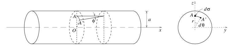
Figure 1: Torsion of a circular cylinder
