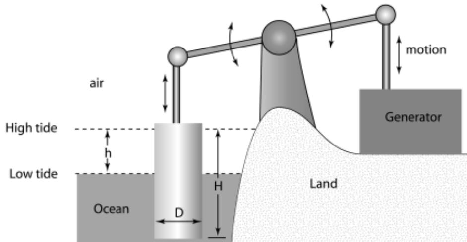
An inventor proposes to generate power from the tidal rise and fall of the ocean surface by linking a float to an electric generator. The proposed device is sketched in the figure above. A cylindrical tank of diameter  $D = 20$  m and height  $H = 15$  m is attached to a lever that causes the armature of an electric generator to rotate as the tank rises and falls with the level of the ocean. The density of ocean water is  $\rho = 1030$  kg/m<sup>3</sup>.
