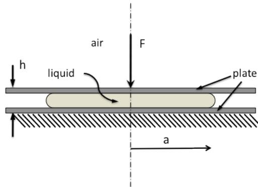
A drop of liquid of volume  $V$  is squeezed between two parallel smooth surfaces. These surfaces are non-wetting to the liquid (for example consider mercury being squeezed between two glass slides). The liquid is squeezed until the thickness of the liquid layer  $t$  is very small compared to the radius  $a$  of the liquid. The three phase contact angle is  $\theta$  and liquid-air surface tension is  $\sigma$ . Gravity effects can be neglected.
