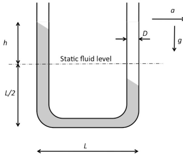
(a) Here we will show how a U-tube filled with liquid can be used to make a cheap accelerometer. Consider a U-tube filled with a liquid density  $\rho$  as shown in the above figure. The U-tube is being accelerated to the right at  $a \text{ m/s}^2$ . Express the acceleration  $a$  in terms of the height  $h$  the fluid reaches above static level in the left leg and other geometric parameters of the tube.
