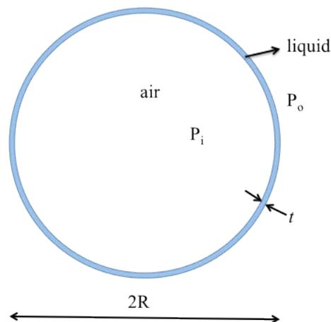
Consider a soap bubble of radius  $R$  and film thickness  $t$  as shown above. The liquid-air surface tension is  $\sigma$  and density of the liquid is  $\rho$ . What is the pressure  $P_i$  inside the soap bubble if the outside pressure is  $P_o$ ?
