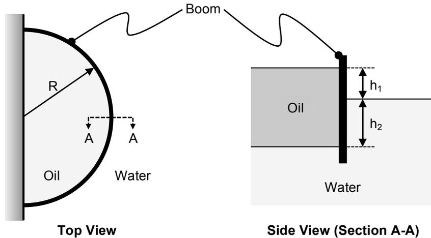
Consider a semi-circular boom of radius  $R$  that is deployed to contain oil spill near a dock as shown above. The boom floats on the water and acts as barrier for the spreading oil. The oil has a density  $\rho_o$  and water has density  $\rho_w$  ( $\rho_o < \rho_w$ ). If a volume  $V$  of the oil is spilled, calculate:
