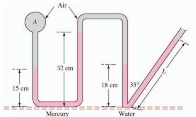
The system above is open to atmospheric pressure ( $10^5$  Pa) on its right side.
