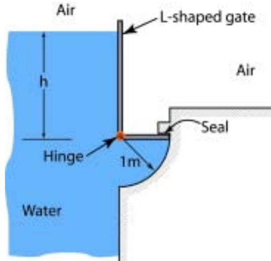
An L-shaped gate can rotate about a hinge pin located at its vertex as shown in the figure above. As the water rises, the depth of the hinge pin,  $h$ , will reach a critical height  $h_c$  and the gate will open. If the length of the lower horizontal arm is 1 m, please find the critical height  $h_c$ . (Please neglect the weight of the gate.)
