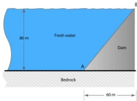
A concrete dam ( $\rho_{\text{concrete}}=2500 \text{ kg/m}^3$ ) of triangular cross-section spans 100 m into the page (i.e., the wetted-area of the dam is  $100 \text{ m}$  (the length of AB)  $\times$   $100 \text{ m}$  (the width into the page) ) in a reservoir as shown above.
