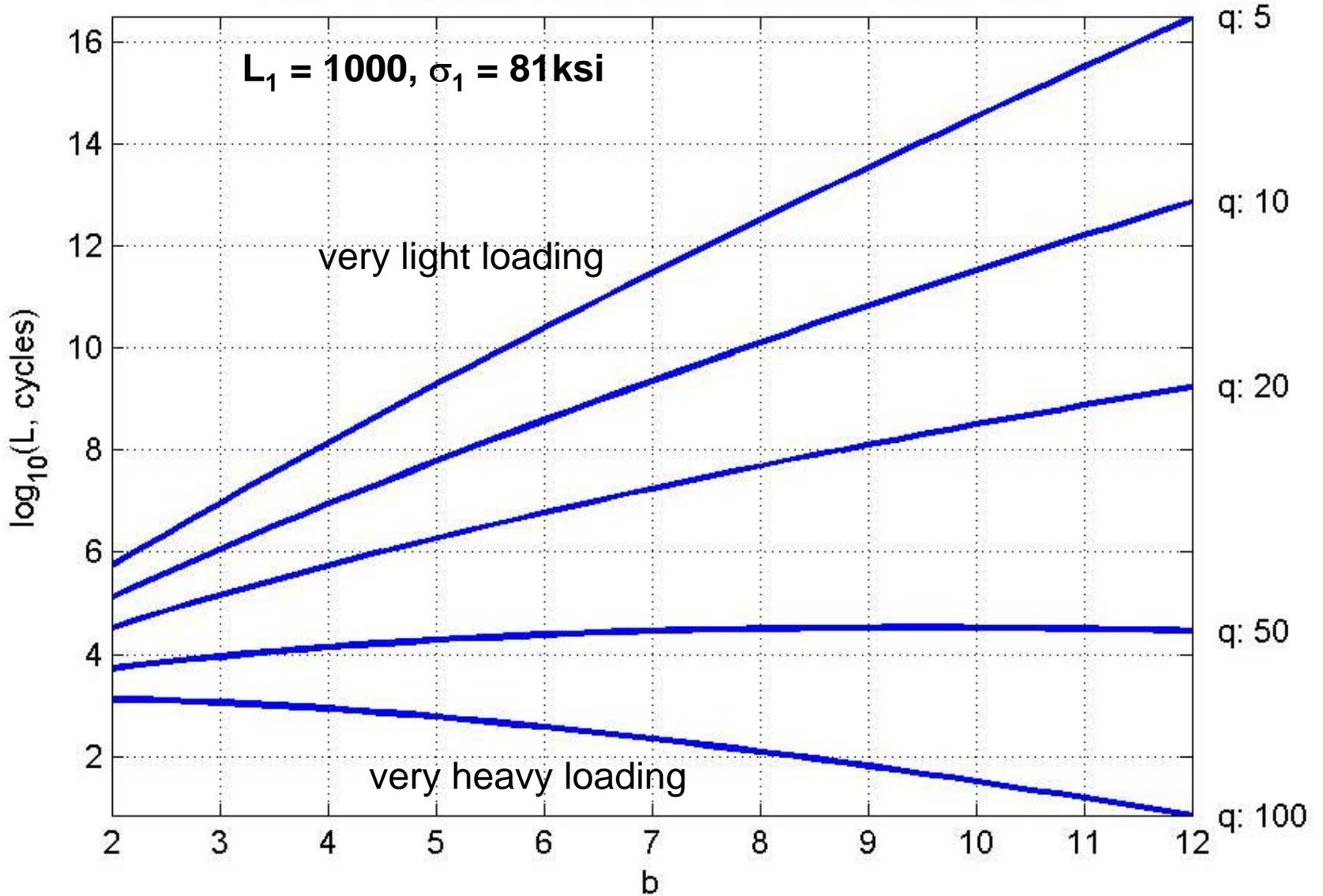
q: twice the standard deviation of the underlying Gaussian stress
