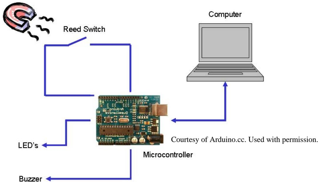
**Figure 1. Schematic of the Arduino security system**
