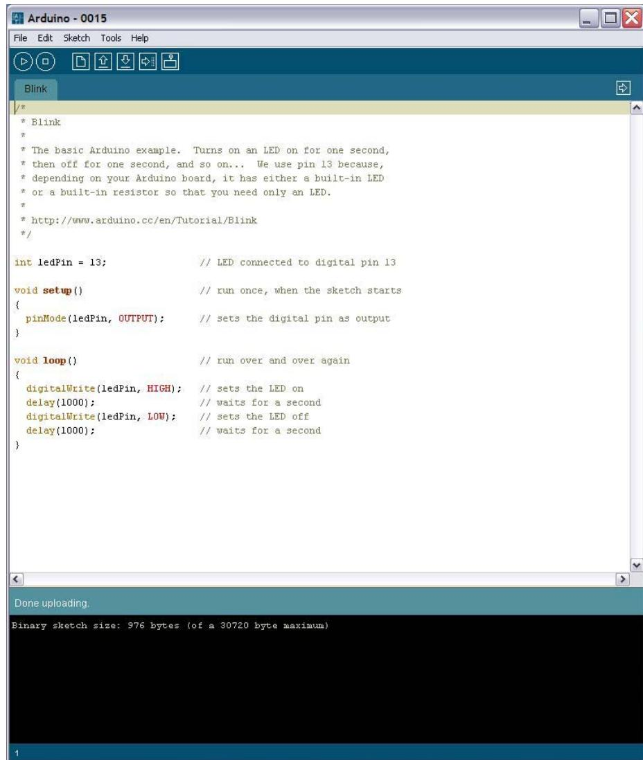
**Figure 2. Arduino software development environment**
