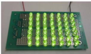
Figure 13: Working LED Light Bank
