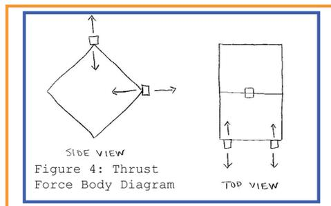
Figure 4: Thrust Force Body Diagram
