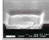
Photo 1 . Cracking of sol-gel deposited PZT after 650C firing
