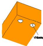
After the ejection by the ejector pin, the surface of the ejected part or surrounding part turns white. When some portion of the part is hard to remove from the mold, that portion also turns white.
