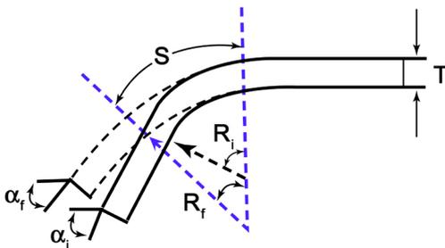
Figure 1: schematic of springback bending
