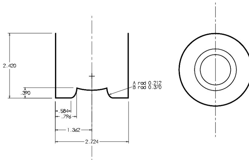
Figure 1: Thermoformed part
