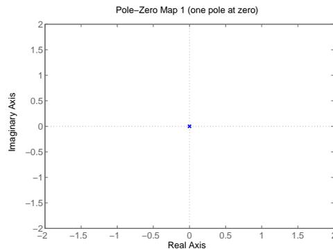
This system has a pole at  $s = 0$ , its transfer function will be
