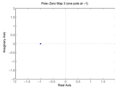
This system has a pole at  $s = -1$ , the transfer function will be
