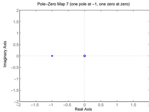
The system has a pole at  $s = -1$  and a zero at  $s = 0$ . The transfer function will be
