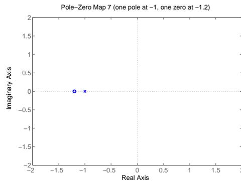
This system has a pole  $s = -1$  and a zero at  $s = -1.2$ . The transfer function will be
