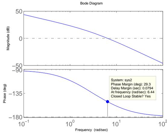
the phase margin is  $29.3^\circ$ . The damping ratio  $\zeta$  is 0.25. Using the same method in question (2), the closed-loop bandwidth  $\omega_{WB} = 10$  (rad/s). Thus
