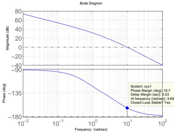
the phase margin is  $16.7^\circ$ . The damping ratio  $\zeta$  is approximately 0.15. Using the same method in question (2), the closed-loop bandwidth  $\omega_{WB} = 14$  (rad/s). Thus
