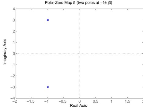
This system has a pair of complex poles at  $s = -1 \pm j3$ . The transfer function will be
