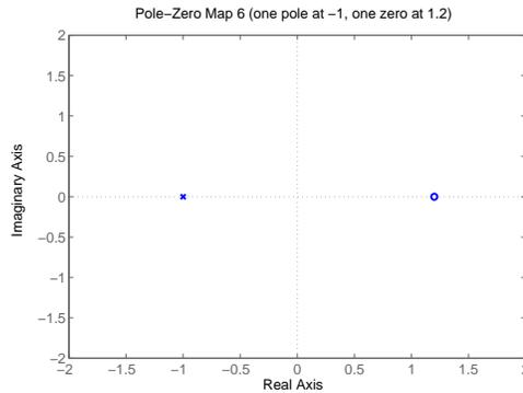
This system has a pole at  $s = -1$  and a zero at  $s = 1.2$ . The transfer
