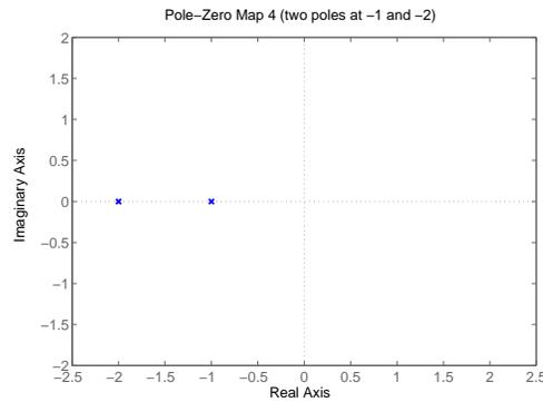
This system has two poles at  $s = -1$  and  $s = -2$ . The transfer function will be
