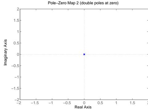
Because this system has double poles at  $s = 0$ , the transfer function will be
