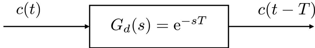
Delay element (or “delay line”)
