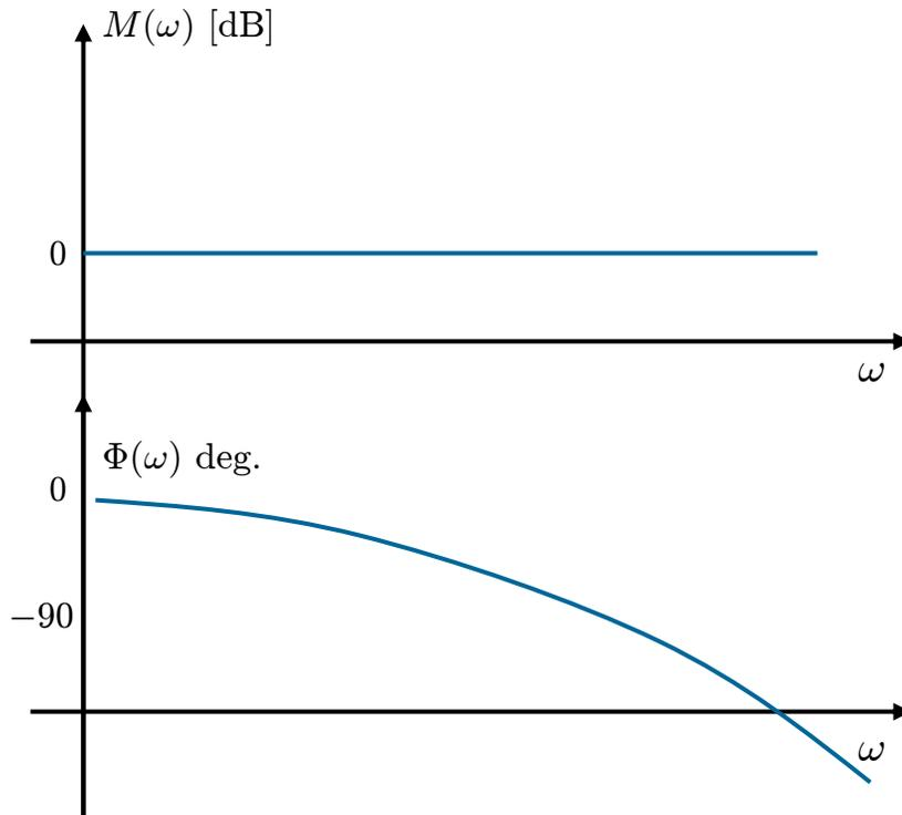
Time delay reduces the phase margin; therefore time delay results in reduced stability
