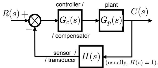
purpose: to improve the system's dynamics by proper choice of the controller TF and gain
