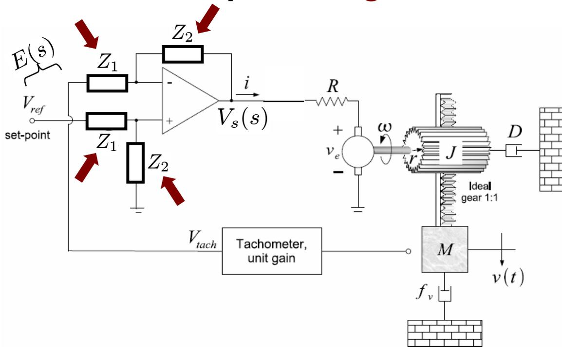
Input-output relation of differential amplifier with general impedances
