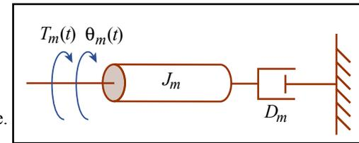
Assume an equivalent load of inertia  $J_m$  and damping  $D_m$ , subject to the motor's torque  $T_m(s)$ .
