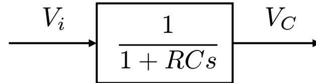
We recognize the voltage divider configuration, with the voltage across the capacitor as output. The transfer function is obtained as
