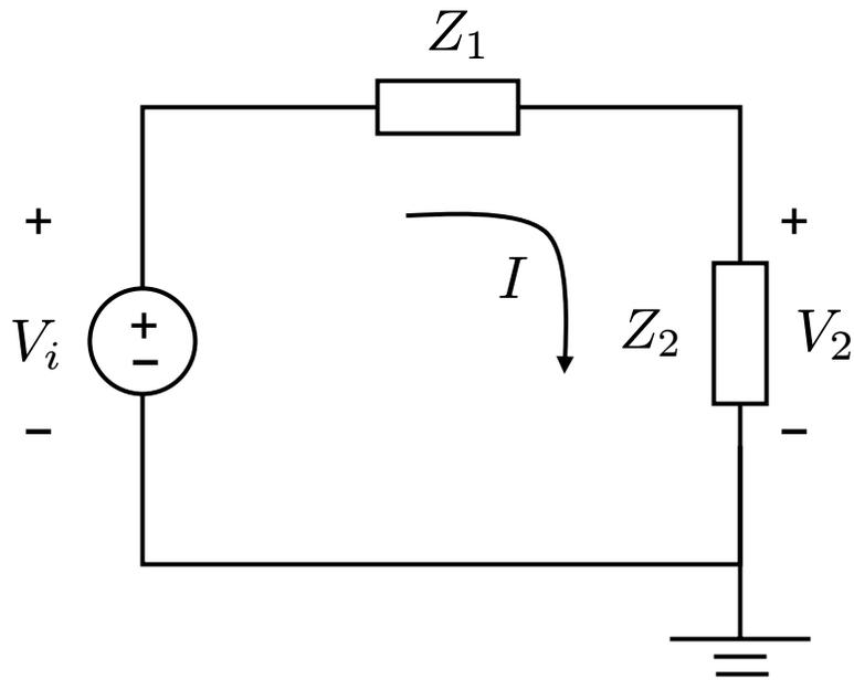
Equivalent circuit for computing the current  $I$ .
