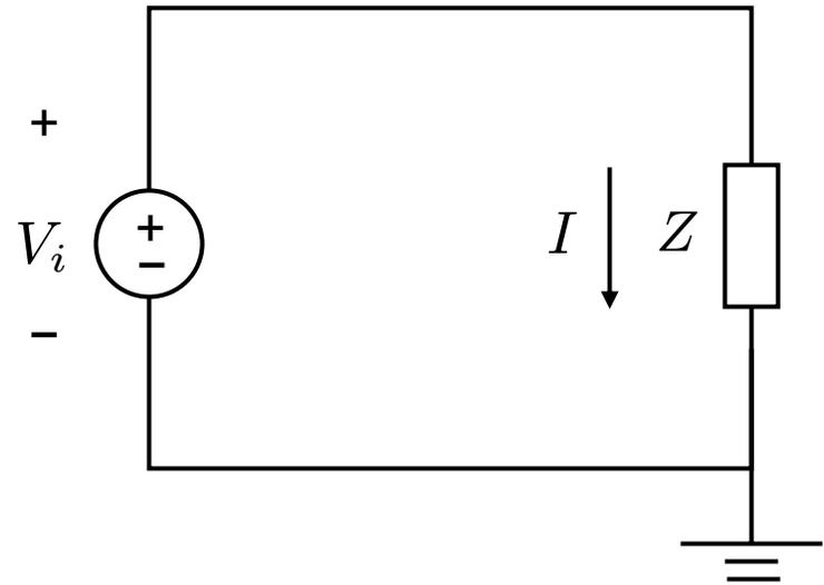
Since the two impedances are in series, they combine to an equivalent impedance
