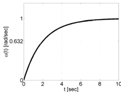
$$J\dot{\omega} + b\omega = T_0u(t), \quad \omega(0) = \omega_0 \quad \Rightarrow$$
