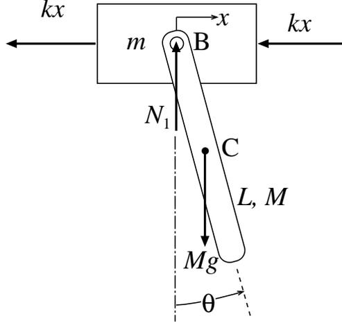
Figure 3: Free-body diagram of carriage plus pendulum.
