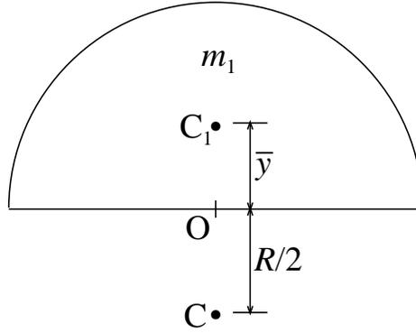
Figure 2:  $I_1$  is the moment of inertia of the semicircular part about C.
