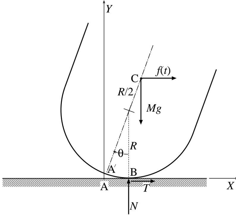
Figure 4: Free-body diagram of rocker rolling without slip.
