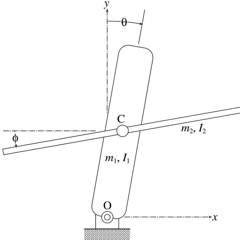
Figure 4: Mechanical model of tight-rope walker.
