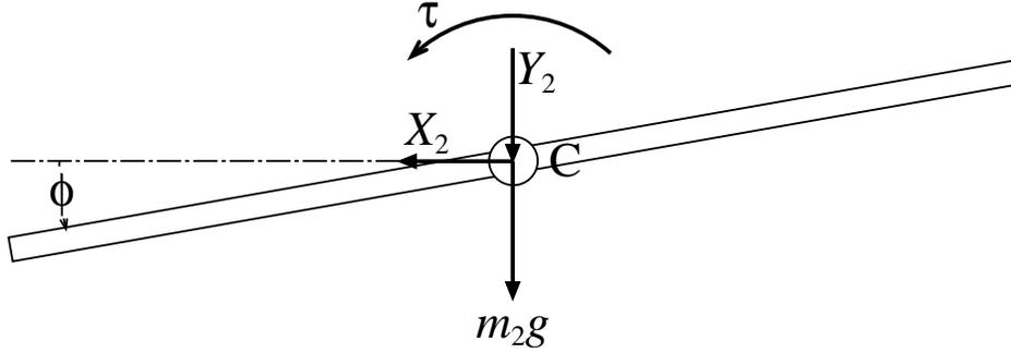
Figure 6: Free body diagram of balancing pole.
