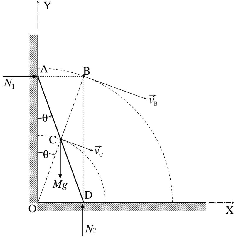
Figure 2: Study of the motions of points C and B.
