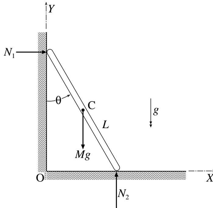
Figure 1: Free-body diagram with generalized coordinate  $\theta$ .
