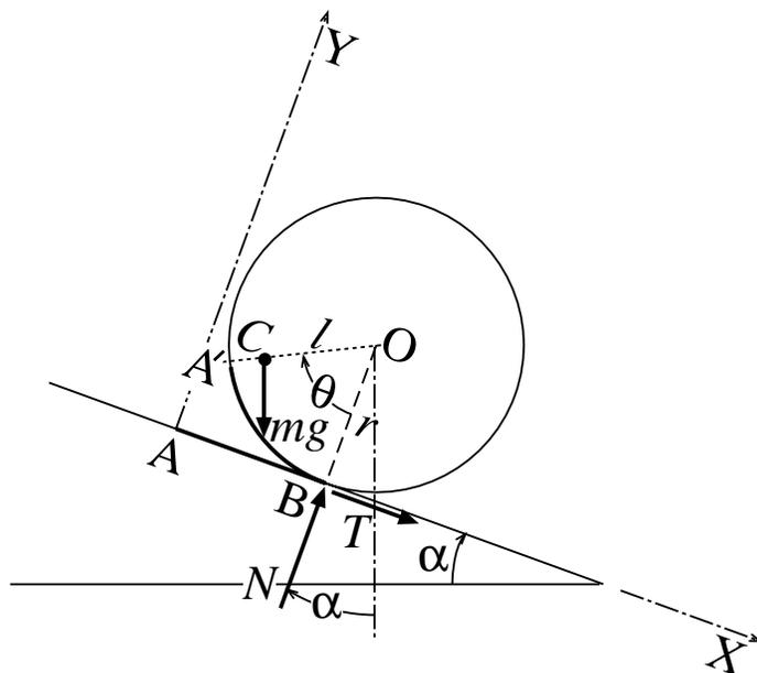
Figure 3: Free body diagram of disk rolling down incline.
