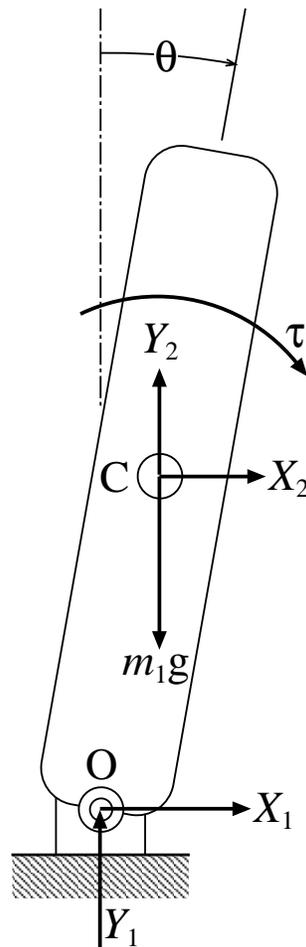
Figure 5: Free body diagram of performer model.
