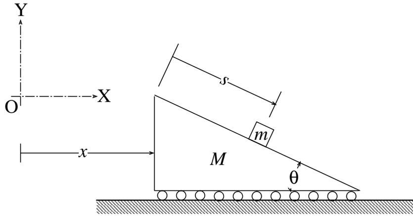
Figure 1: Mass  $m$  slides down inclined plane of mass  $M$ .
