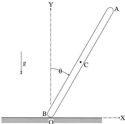
Figure 4: Rod of mass  $m$  and length  $L$  slides on floor as it falls.
