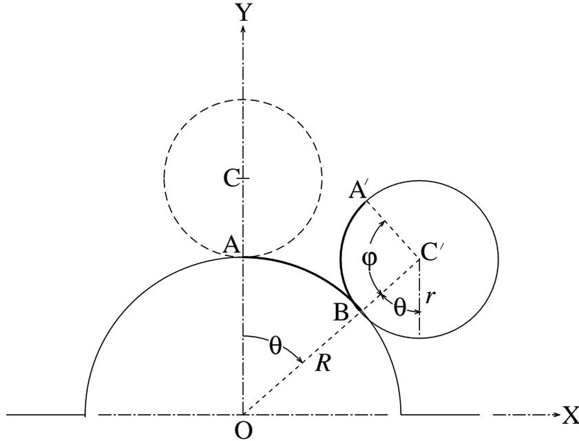
Figure 3: Disk of radius  $r$  rolls on fixed cylindrical surface of radius  $R$ .
