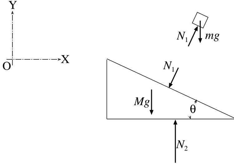
Figure 2: Forces acting on particle  $m$  and inclined plane  $M$ .
