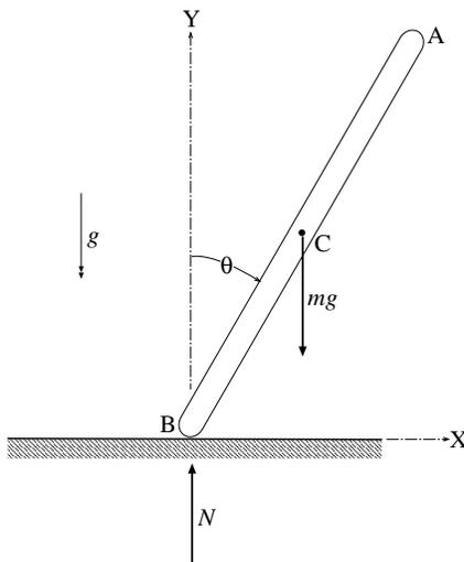
Figure 5: Rod is acted on by gravity force  $mg$  and floor reaction  $N$ .
