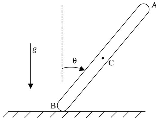
Figure 1: Rod falls under the influence of gravity
