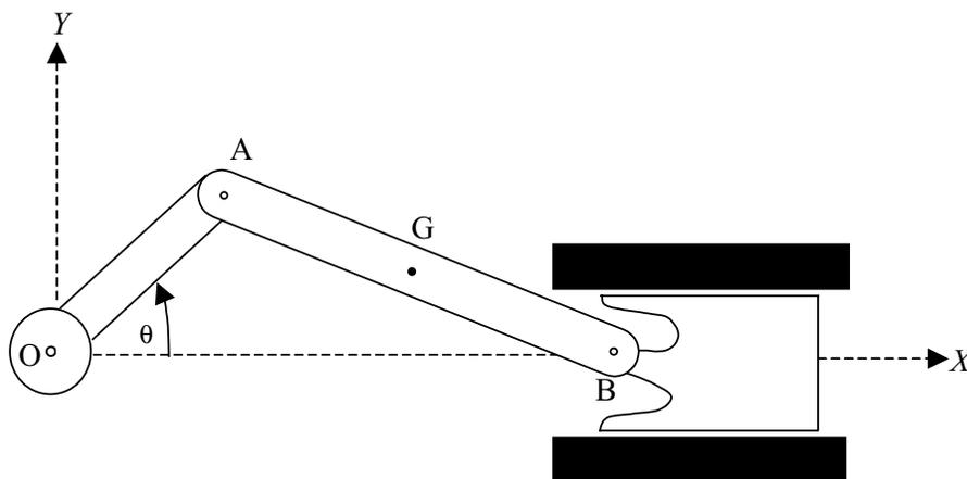
In the mechanism shown let the length of the crank throw  $OA$  be  $a$  and length of the connecting rod  $AB$  be  $2a$ . The point  $G$  is at the midpoint of the connecting rod  $AB$ .
