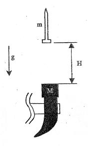
We hold the hammer, upside down, in one hand and carefully drop the nail from a height H and measure its rebound height h. This is fairly tricky as the nail must be dropped perfectly vertical. After several trials the average value of the ratio h/H is found to be 0.1. Use this result to obtain an estimate of the coefficient of restitution e. Then derive a second equation relating the velocities  $v_1$  and  $V_1$  to the initial hammer head velocity  $V_0$ .
