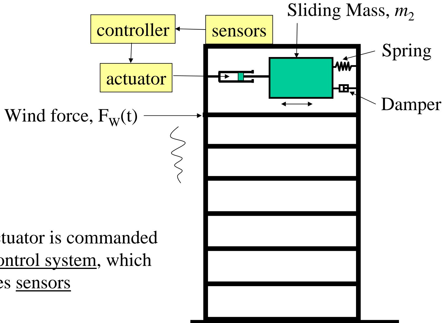
The actuator is commanded by a control system, which requires sensors
