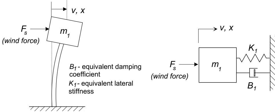
This simplified model is the classic parallel mass-spring-dashpot system, excited by an external force  $F_s$ , and has a transfer function relating the velocity  $v$  to the force
