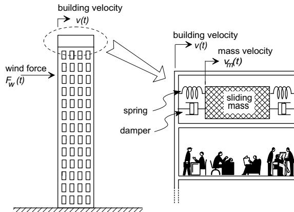
In the final three lab sessions you will design and implement an active damping system and test it on a model building. To prepare for this project we will develop linear models of the building with a damper in this assignment, and you will use the results as the basis for your control system design in the lab.
