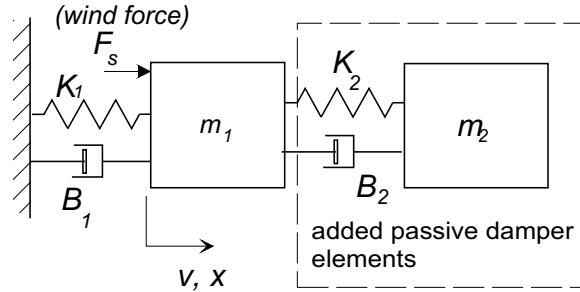
The values of  $m_2$ ,  $B_2$ , and  $K_2$  are chosen so that the motions of the two masses are *out-of-phase*, that is when  $m_1$  is travelling to the right  $m_2$  is travelling to the left. The forces transmitted through  $K_2$  and  $B_2$  act to inhibit the motion of  $m_1$ . Effective reduction of the motion requires careful “tuning” of the elements.
