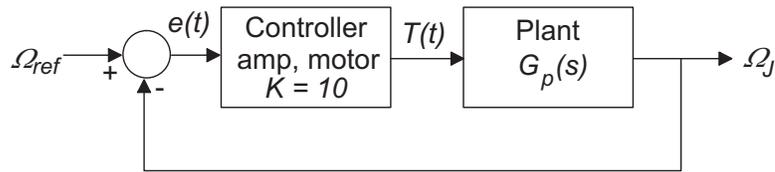
$$\text{Closed Loop : } G_p(s) = \frac{\Omega_1(s)}{T_s(s)} = \frac{K_r}{BJs^2 + (B^2 + K_r J)s + 2K_r B} = \frac{1.019 \times 10^4}{0.0310s^2 + 3159s + 2037}$$
