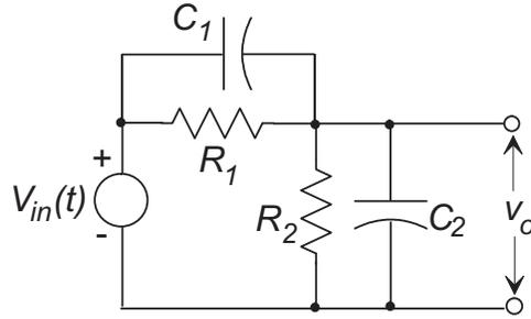
$$\text{Voltage Divider : } \frac{V_o(s)}{V_{in}(s)} = \frac{(Z_{R_2} || Z_{C_2})}{(Z_{R_1} || Z_{C_1}) + (Z_{R_2} || Z_{C_2})}$$
