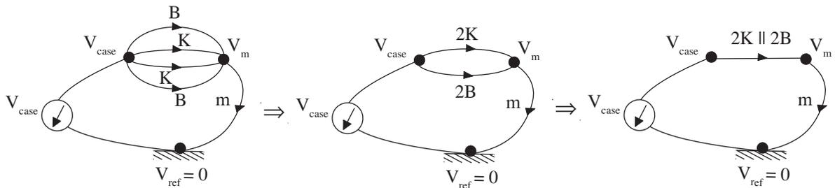
(b) There are two independent energy storage elements: one is the mass inertia (requiring to know  $V_m$ ) and the other is the spring (requiring to know  $x_m - x_{case}$ ). The two springs act in parallel and are dependent.
