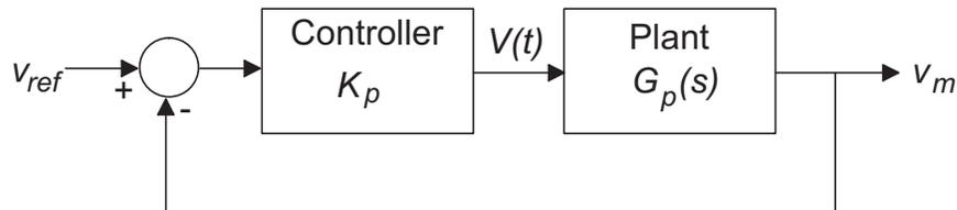
$$\frac{V_m(s)}{V_{ref}(s)} = \frac{K_p G_p(s)}{1 + K_p G_p(s)} = \frac{K_p B}{ms + (1 + K_p)B}$$
