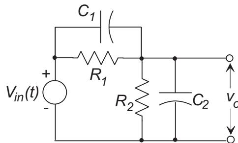
Now suppose  $R_1 = 50 \text{ k}\Omega$ ,  $C_1 = 1 \mu\text{fd}$ ,  $R_2 = 100 \text{ k}\Omega$ ,  $C_2 = 0.5 \mu\text{fd}$ . Evaluate the transfer function with these values, and write the differential equation in this case. Can you explain what has happened to the order of the system?
