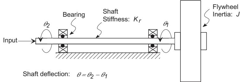
The torsional stiffness of a cylindrical shaft of diameter  $D$  and length  $l$  is
