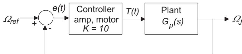
Use MATLAB's `feedback()` function (see the handout) to find the closed-loop transfer function. As in part (c), plot the step response, and estimate the closed-loop rise time.
