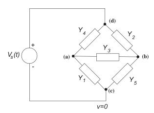
(b) KCL equations for node (a) and (b) are derived. Note that  $I_{\overrightarrow{ab}}$  stands for the current in branch ab from (a) toward (b).
