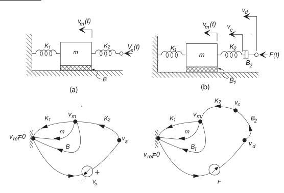
(a) The linear graph models of the system are shown in the above figure. We write the KCL for node (m) and then substitute for admittances. The positive sign for current (force) corresponds to the current out of a node:
