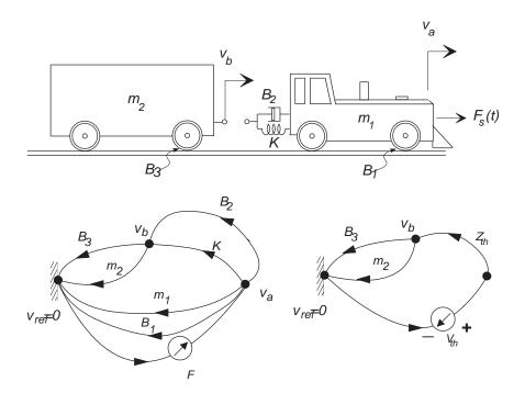
(a) The linear graph model of the system is shown above. The locomotive section is equivalently represented by a Thévenin source and impedance. The Thévenin impedance is computed by removing the force (current) source and looking to the system from node (b) and (ref):
