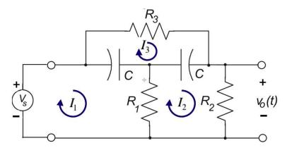
$$\begin{cases} \text{Loop 1:} & -V_s + \frac{1}{Cs}(I_1 - I_3) + R_1(I_1 - I_2) = 0 \\ \text{Loop 2:} & R_1(I_2 - I_1) + \frac{1}{Cs}(I_2 - I_3) + R_2I_2 = 0 \\ \text{Loop 3:} & \frac{1}{Cs}(I_3 - I_1) + R_3I_3 + \frac{1}{Cs}(I_3 - I_2) = 0 \end{cases}$$
