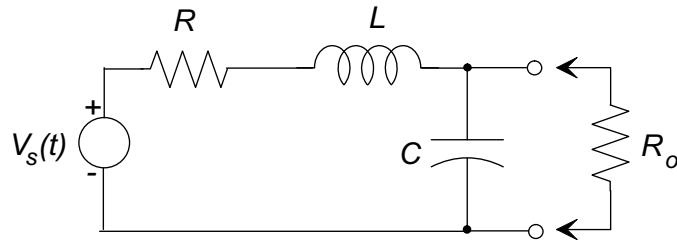
**Problem 5:** Does the input impedance uniquely characterize a system? Answer the question by determining the input impedance of the two electrical circuits below:
