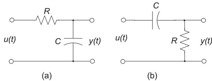
(a) Transfer functions can be simply calculated by utilizing the voltage divider rule:
