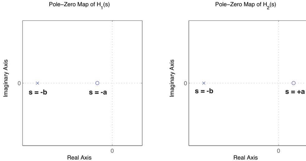
Both systems have the same magnitude plot ( $|H_1(j\omega)| = |H_2(j\omega)|$ ), while they differ on the phase plot:
