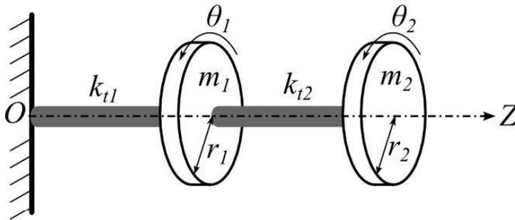
Figure 1: Torsional oscillator
