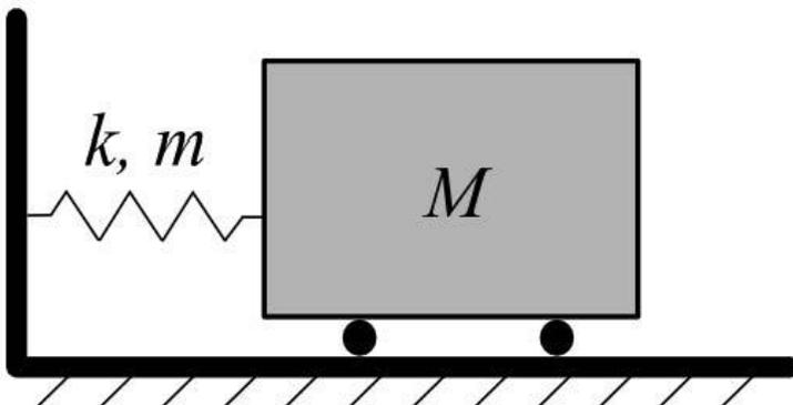
Hint: Compute the kinetic energy of the system and account for the kinetic energy of the spring. Note that the velocity of the spring varies from zero at the point of attachment to the wall to  $\dot{x}$  at the point of attachment to the moving
