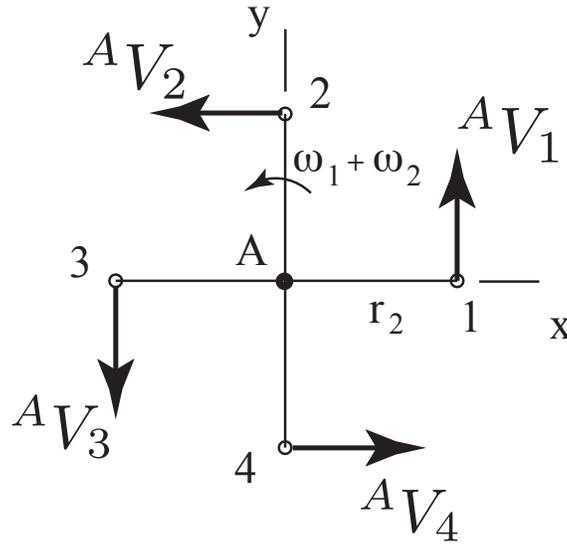
$${}^A V_1 = r_2(\omega_1 + \omega_2)[\hat{j}] \quad {}^A V_2 = r_2(\omega_1 + \omega_2)[-\hat{i}] \quad {}^A V_3 = r_2(\omega_1 + \omega_2)[-\hat{j}] \quad {}^A V_4 = r_2(\omega_1 + \omega_2)[\hat{i}]$$
