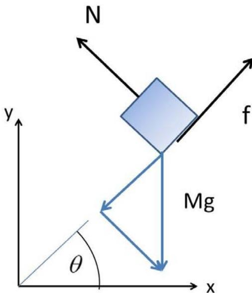
b. The free body diagram is on the left. In the direction tangent to the slope the mass times the acceleration must be equal to the sum of the friction force and the tangential component of the gravitational force on the box. This is worked out in the equations below.
