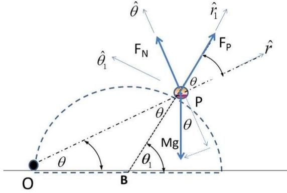
Using polar coordinates with origin at point B,  $\mathbf{V}_{P/O}$  and  $\mathbf{a}_{P/O}$  are easily obtained.
