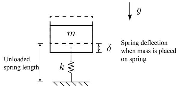
When a mass is placed on the spring, in the presence of gravity, the spring deflects due to the mass's weight.
