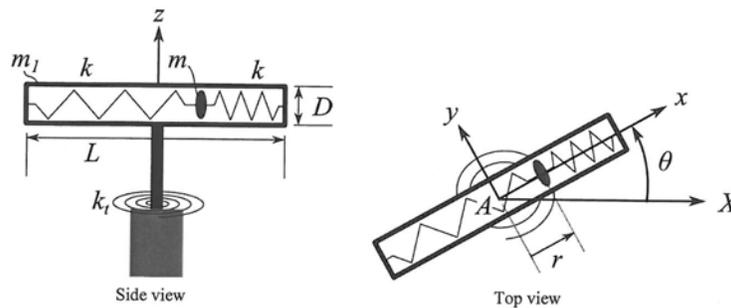
$(\theta, r)$  defined on the top view of the figure form a set of complete and generalized coordinates, which describe this two degree of freedom system. You should not assume that  $(\theta, r)$  or their first two time derivatives are zero.
