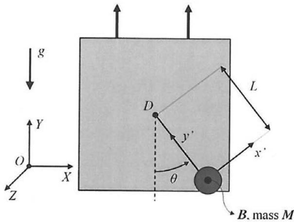
The elevator has velocity  $\dot{Y}$  and acceleration  $\ddot{Y}$ . Their values are given and therefore 'Y' does not have to be considered an independent degree of freedom, because it is constrained to fixed values. The elevator is also not allowed to move in the X or Z directions. This is a planar motion problem, requiring one independent coordinate,  $\theta$ , as shown in the figure to the left.
