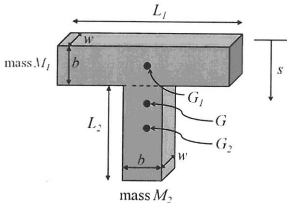
a). Find the location of the center of mass of the combined object, which lies somewhere on the vertical line which passes through  $G_1$  and  $G_2$ . Express it as a distance “s” measured from the top of the “T”, as shown in the figure.
