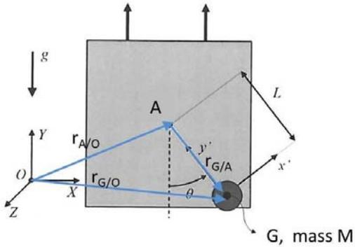
a). In the figure above the point D is the point about which the angular momentum is to be computed. Hence D=A in equations (1) and (2). The point labeled 'B' in the figure is the center of mass for the rigid body and therefore B=G in equations (1) and (2). These are shown in the figure to the left. The rigid body in this case is the combination of the massless pendulum arm and the concentrated mass, M. Also shown in the figure are the position vectors which satisfy the
