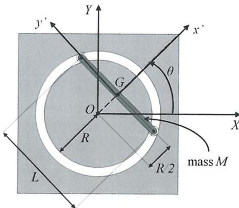
friction. Neglect the mass of the rollers. The radius of the track is  $R$  and  $L = \sqrt{3}R$ . Find an equation of motion of the rod as a function of the coordinate,  $\theta$ , as shown in the figure. The frame  $Gx''y''z''$  is fixed to the center of mass of the rod.
