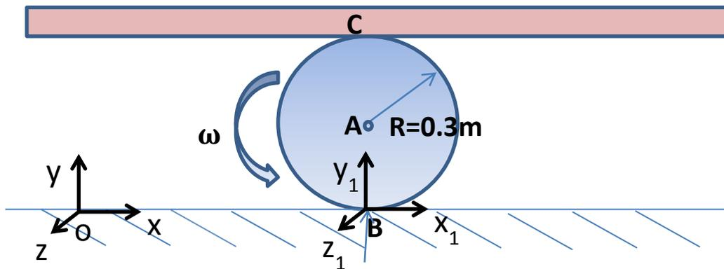
This problem is solved by using the standard form of the velocity equation for a point on a translating and rotating rigid body. The standard velocity equation is given below and defined carefully one time in this first problem set.
