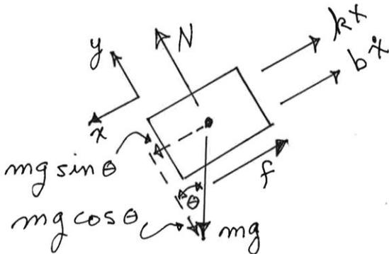
Next sum forces in the x direction and equate them to the mass times acceleration in the x direction. This leads to the following equation of motion. Note that the spring, damper and friction forces are all preceded by minus signs, because they are drawn on the fbd in the negative x direction, given the assumption that the displacement and velocity were assumed to be positive.
