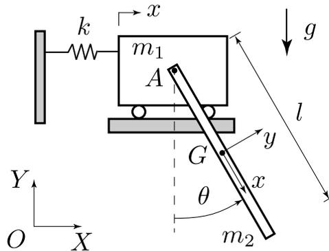
Derive the equations of motion for this system by Lagrange. Specifically,
