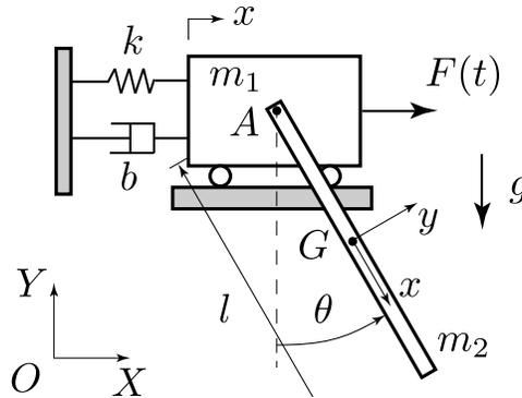
Derive the equations of motion for this system **by Lagrange**. Specifically, show the generalized forces.
