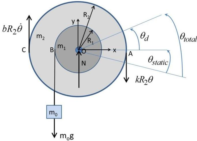
virtual work done in a virtual rotation  $\delta\theta_d$  can be figured out by inspection. The only external non-conservative moment doing work during a rotation is due to the dashpot. A positive rotational velocity results in a torque given by  $\vec{\tau}_{dashpot} = -bR_2^2 \dot{\theta}_d \hat{k}$ . The work done in a positive rotation  $\delta\theta$  is given by
