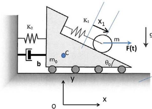
The disk is restrained by a spring,  $K_1$ , attached at one end to the cart. The other end of the spring attaches to an axel passing through the center of the disk. The cart is also attached to a wall by a spring of constant,  $K_2$ , and a dashpot with constant 'b'. An horizontal external force,  $F(t)$ , is applied at the center of mass of the disk as shown.
