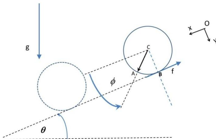
a). Assume that the wheel does not slip as it rolls down the hill. Derive the equation of motion using Lagrange equations.
