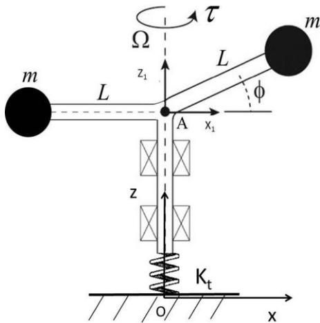
The shaft rotates with a time varying angular velocity  $\Omega$  with respect to the  $O_{xyz}$  inertial frame. The arms are of length  $L$ . The frame  $A_{x_1y_1z_1}$  rotates with the arms and attached masses. A time varying torque is applied to the rotor about the  $z$  axis, such that  $\tau_{/A} = \tau_o(t)\hat{k}$ . Note that the angle  $\phi$  is fixed.
