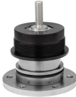
The figure above shows a commercial vibration isolation bearing. It combines a spring and damper in a single device. You use it by placing one or more of them under the device that you wish to isolate from vertical motion of the floor on which it sits. A diagram is provided showing the equivalent model of the microscope sitting on the bench with these bearings installed. The floor is vibrating in the vertical direction at a frequency of 10 Hz.
