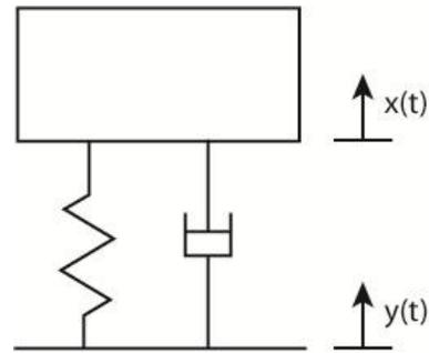
In this case four bearings support the lab bench as shown. One is attached to each corner of the bench. The microscope and bench sitting on the bearings is equivalent to the one dimensional mass-spring-damper system, as shown on the right. The mass of the bench plus microscope is such that the natural frequency of the bench sitting on the bearings is 3.0 Hz. The manufacturer claims that it has been designed to provide a damping ratio for vertical motion of 13%.
