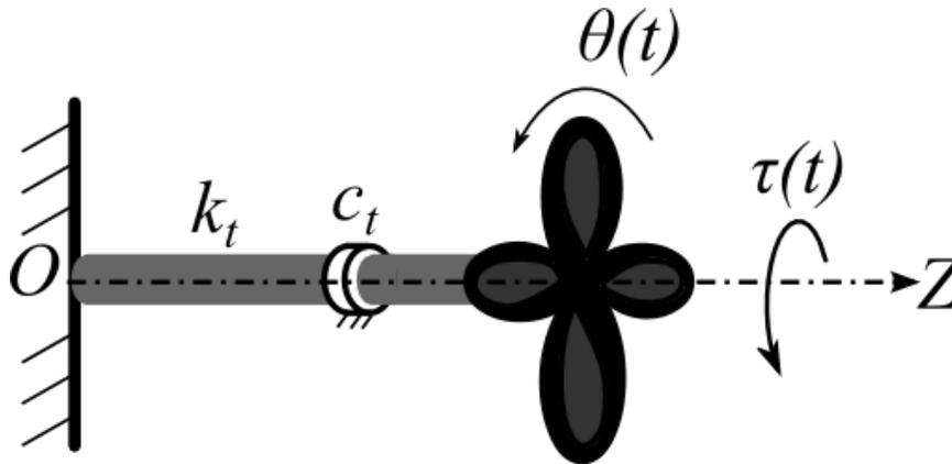
Since the system is linear, the constant rate rotation at 45 RPM may be separated from the oscillatory motion of the propeller, which results from the oscillatory torque. Thus the constant rate rotation may be neglected in the analysis of the response to the oscillatory torque.
