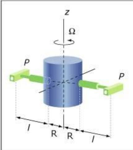
**Concept Question:** Does the total angular momentum of the satellite change as a result of the extension of the booms supporting the experiment modules. Assume the angular momentum is computed with respect to the center of mass of the satellite?
