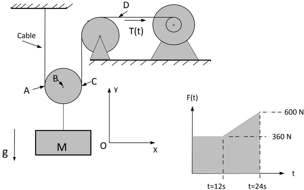
**Concept question:** Do you expect the speed of the mass to be constant while the force is constant during the interval 0 to 12 seconds? (a) Yes (b) No (c) I don't know what principle to apply.
