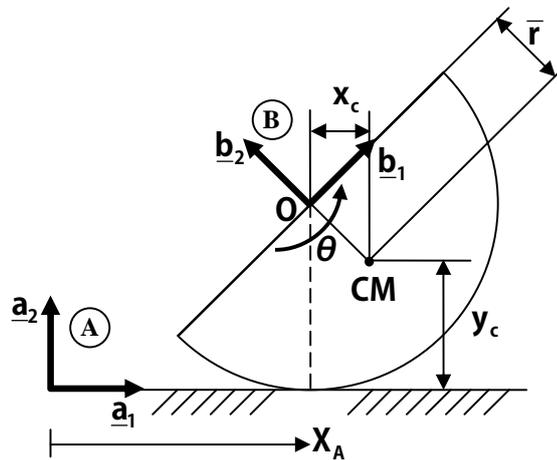
Rolling half-disk has only one degree of freedom with the constraint of  ${}^A \underline{v}^O = r\dot{\theta}$ .
