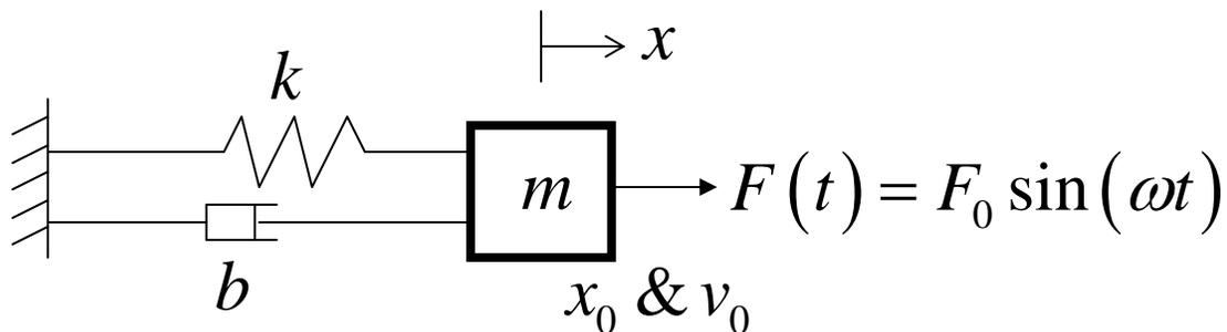
A mass-spring-damper system is subject to an external sinusoidal force  $F(t)$  with amplitude  $F_0$ , and angular frequency  $\omega$ . The position of particle,  $x$ , is zero when the spring is neither compressed or stretched. The mass of the particle is  $m$ , the damping coefficient is  $b$  and the spring constant is  $k$ . Initial condition is expressed as  $x(0) = x_0$  and  $v(0) = v_0$ . Derive the equation of motion for this mass-spring-damper system.
