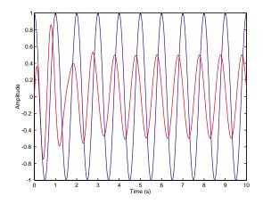
Figure 6: The input time function is a cosinusoid that starts at t = 0. The output of an LTI system with system function  $H(s) = 5s/(s^2 + 2s + 101)$  is shown in red.
