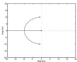
Figure 5: Root-locus plot of the poles of H(s)as K varies for  $G(s) = s/(s^2 + 2s + 101)$ .
