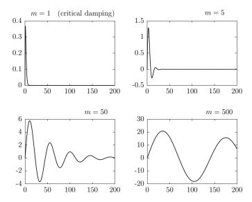
Figure 1.30: Initial condition response  $(x_0 = 0, v_0 = 1)$  for second-order system with k = 1 N/m, b = 2 N-sec/m, and where m takes the values m = 1, 5, 50, 500 kg.
