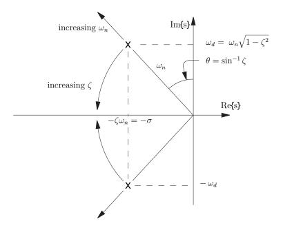
Figure 1.23: Pole locations in the s-plane for second-order mechanical system in the underdamped case  $(0 < \zeta < 1)$ . Arrows show the effect of increasing  $\omega_n$  and  $\zeta$ , respectively.
