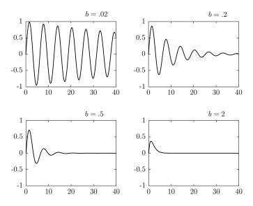
Figure 1.29: Initial condition  $(x_0 = 0, v_0 = 1)$  response for second-order system with m = 1 kg, k = 1 N/m, and four values b = .02, .2, .5, 2 N-sec/m.
