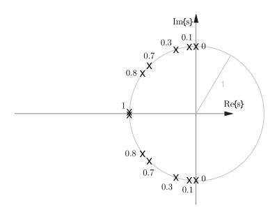
Figure 1.24: Pole locations for  $\omega_n=1$  and  $\zeta=0,0.1,0.3,0.7,0.8,$  and 1.
