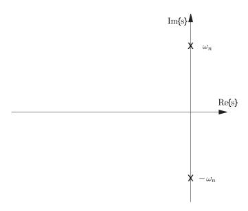
Figure 1.21: Pole locations in the s-plane for second-order mechanical system in the undamped case ( $\zeta=0$ ).
