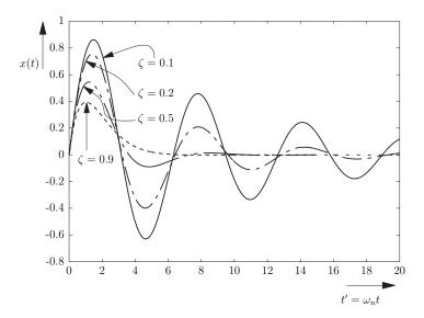
Figure 1.26: Initial condition response for second-order mechanical system in the underdamped case (0 <  $\zeta$  < 1), with varying values of  $\zeta = 0.1, 0.2, 0.5, 0.9$ . Time axis is normalized to  $t' = \omega_n t$ .
