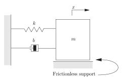
Figure 1.19: Second-order mechanical system.
