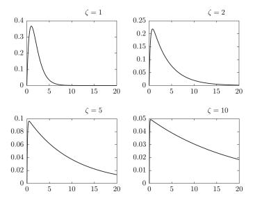
Figure 1.33: Initial condition response for second-order system in the over-damped case, with  $\omega_n = 1$  and  $\zeta = 1, 2, 5, 10$ .
