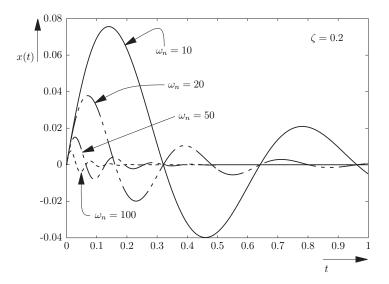
Figure 1.25: Initial condition response  $(x_0=0,\ v_0=1)$  for second-order mechanical system in the underdamped case  $(0<\zeta<1)$ , with varying values of  $\omega_n=10,\ 20,\ 50,\ 100$ , and constant damping ratio  $\zeta=0.2$ .
