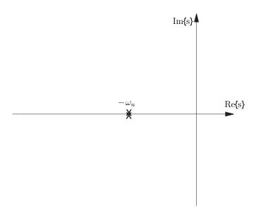
Figure 1.31: Pole locations in the s-plane for second-order mechanical system in the critically-damped case ( $\zeta = 1$ ).
