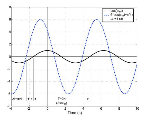
Figure 1.22: Natural response for second-order mechanical system in the undamped case ( $\zeta=0$ ) with M=3 (and thus a peak value of 2M=6) and  $\phi=\pi/4$ . A reference unit amplitude cosine is also shown.
