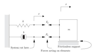
Figure 1.20: Free body diagram for second-order system.
