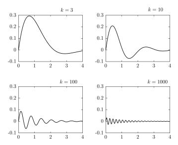
Figure 1.28: Initial condition  $v_0 = 1$  response for second-order system with m = 1 kg, b = 2 N-sec/m, and four values k = 3, 10, 100, 1000 N/m.
