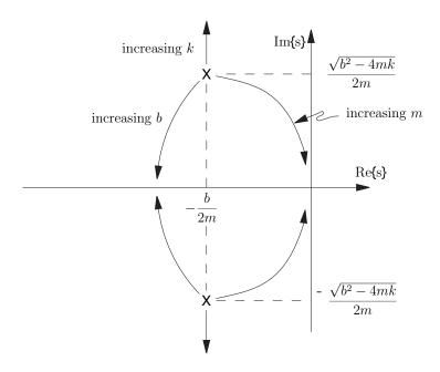
Figure 1.27: Pole locations in the s-plane for second-order mechanical system in the underdamped case (0 <  $\zeta$  < 1). Arrows show the effect of increasing k, b, and m, respectively.
