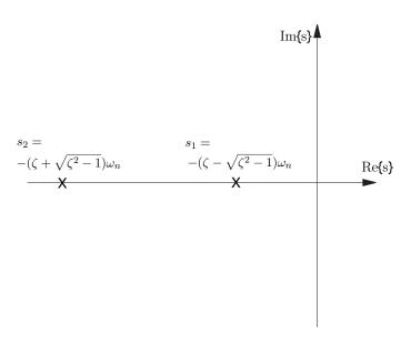
Figure 1.32: Pole locations in the s-plane for second-order mechanical system in the overdamped case ( $\zeta > 1$ ).
