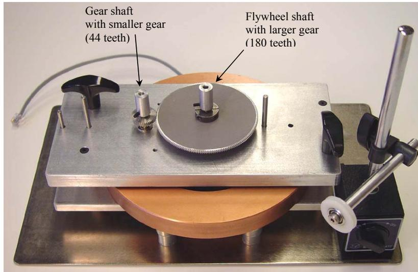
Figure 1: Flywheel apparatus with gear train.
