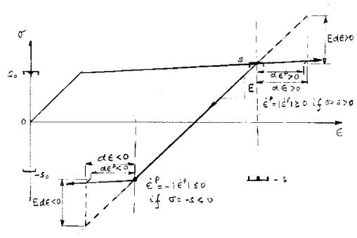
Schematic of plastic loading and unloading from a state of stress which satisfies the yield condition  $f = |\sigma| - s = 0.$
