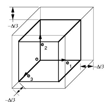
Note that in uniform compaction/dilatation the volume change per unit original volume is given by:
