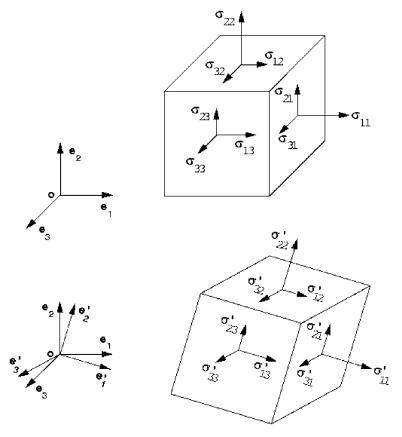
Transformation of stresss components under a rotation of the coordinate system.
