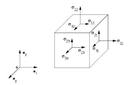
Up till this point, we have considered the components of stress  $\sigma_{ij}$  with respect to a rectangular cartesian coordinate system with origin o and base vectors  $\{e_i\}$ . Let us now consider a second rectangular cartesian coordinate system with the same origin, but a different orthonormal basis  $\{e_i'\}$ ,
