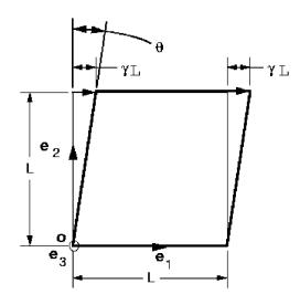
**Pure Shear** with respect to  $(e_1, e_2)$ :
