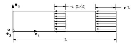
Bodies which experience constant strain are said to be **homogeneously deformed**.
